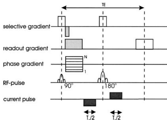
FIGURE 3 Modified spin echo sequence for magnetic resonance current density imaging.
